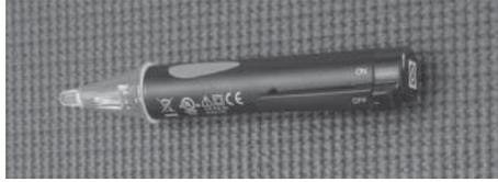
Figure 25 - Non-Contact Circuit Tester
