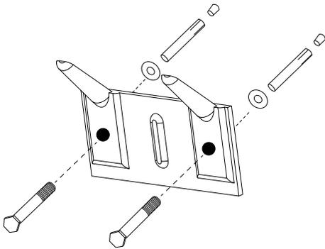
Figure 10 - Mounting Bracket for Masonry Wall.
