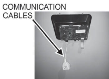
Figure 28. Reconnecting RJ45 Plug from Split Communication Cable
